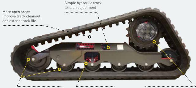
Lifetime sealed and lubricated rollers/idlers reduce maintenance costs
